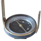
Adjustable Brass Survey Compass Survey Item compass is accurate with a resolution of about 1/2 a degree.
